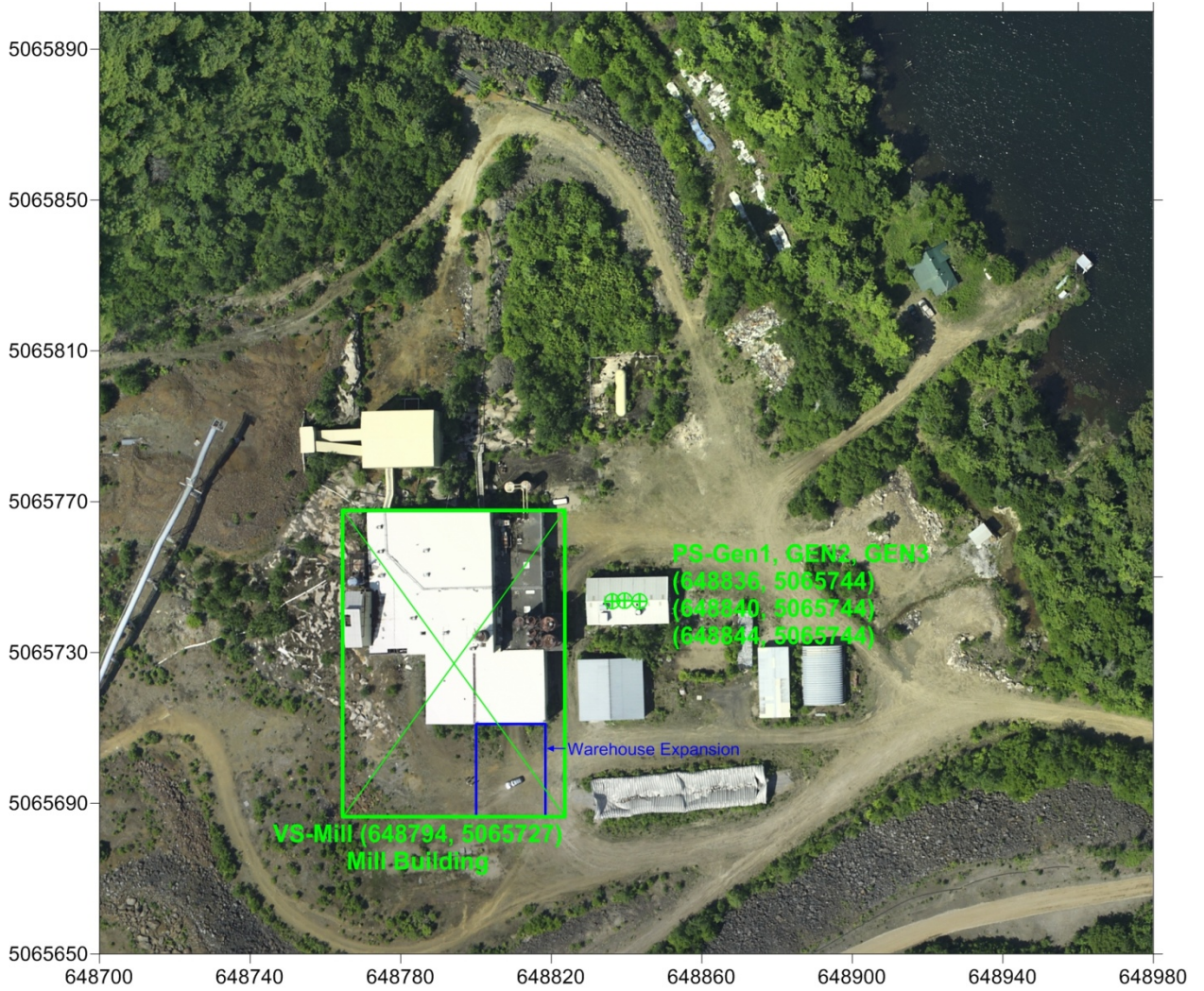
Figure 1- 2 Mill Layout and Emission Sources Locations
